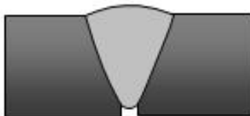
Incomplete root penetration
