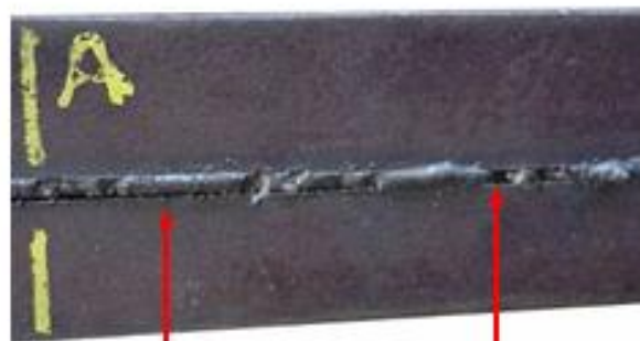
Incomplete root penetration
