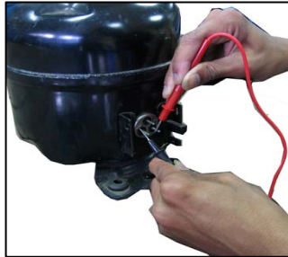
Gambar 5.5 Mengukur kutub/terminal Y-X
