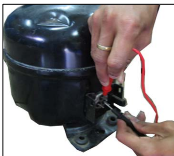
Gambar 5.7 Mengukur kutub/terminal Y-Z
