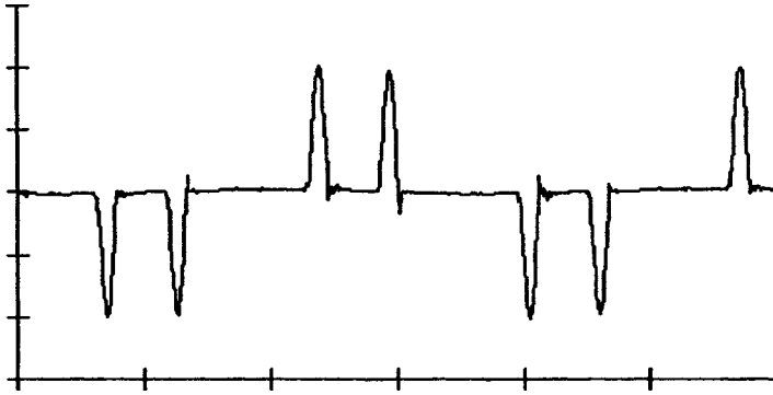
Figure 3.51 Harmonic current waveform of a VSC converter
