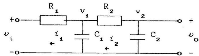
$$\text{Untuk : } R_1 \rightarrow I_{1(s)} = \frac{1}{R_1} [V_i(s) - V_1(s)]$$
