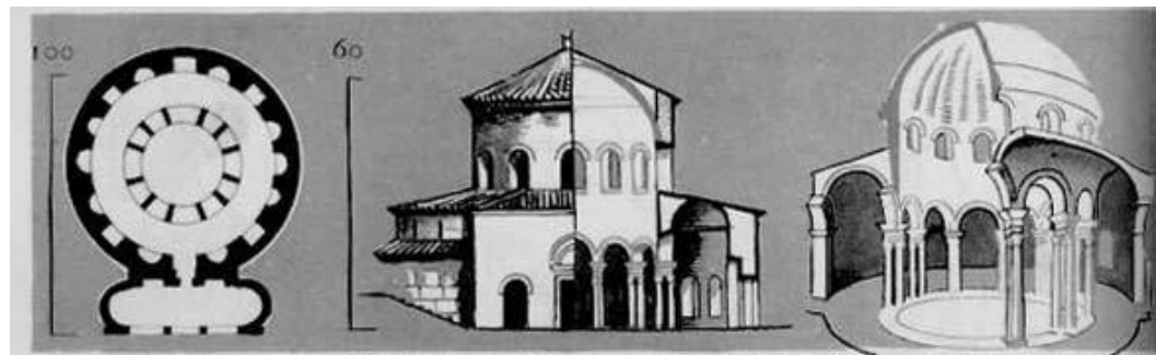
The Mausoleum of S. Costanza, Rome, built by Constantine, c.A.D. 324-329. The dome constructed of concrete with brick ribs and set on a drum supported upon 12 coupled granite columns, the thrust neutralized by the barrel vault of the circular aisle
