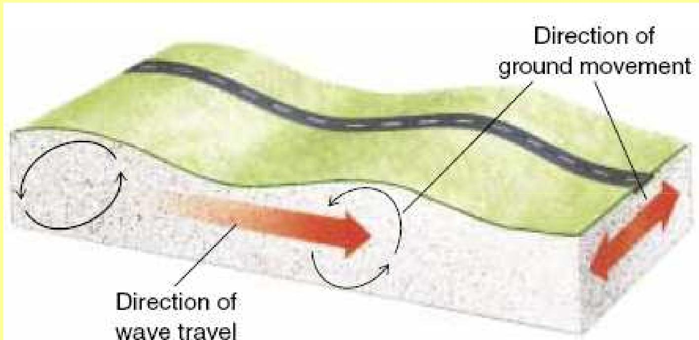
**Figure 10-8** Surface waves. Surface motion includes up-and-down movement like that of an ocean wave and also a side-to-side sway.
