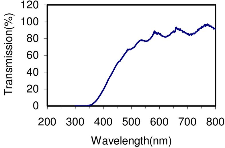
Figure 2. Transmission spectrum of the GaN epilayer.
