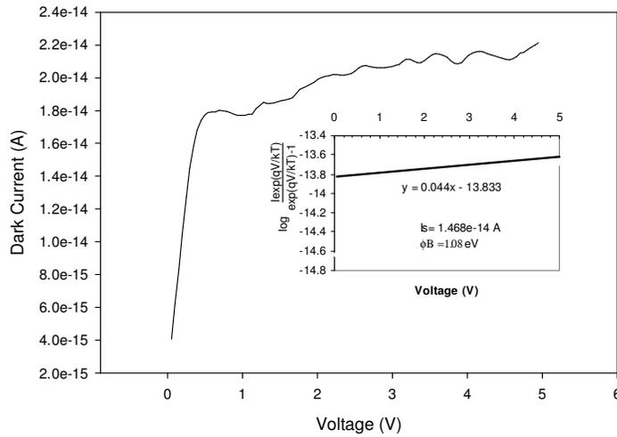
Figure 3. Dark current I-V characteristics for MSM-PD. The inset is logarithmic plot of I vs V
