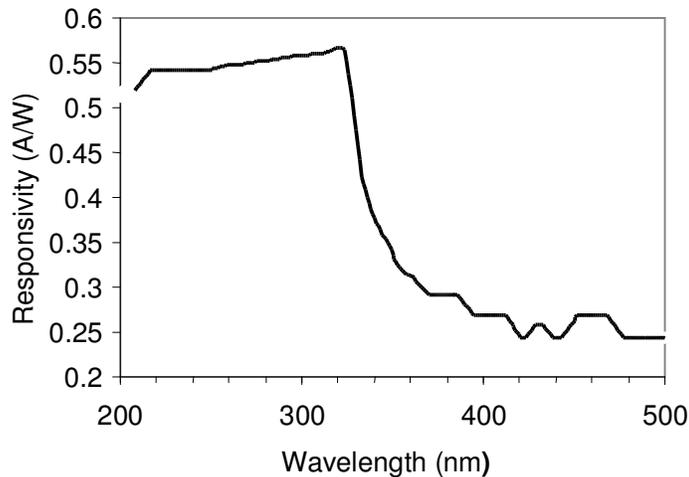
Figure 4. The spectral response of a typical GaN MSM photodetector biased at 2.5 V
