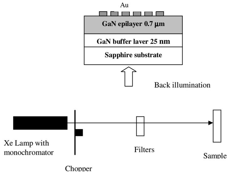
Figure 1. A schematic cross section of the structure and measurement principle of the GaN MSM-PD.
