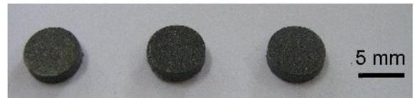
Fig. 2. Visual appearance of typical  $\text{SiO}_2$  Added- $\text{CuF}_2\text{O}_4$  ceramics.
