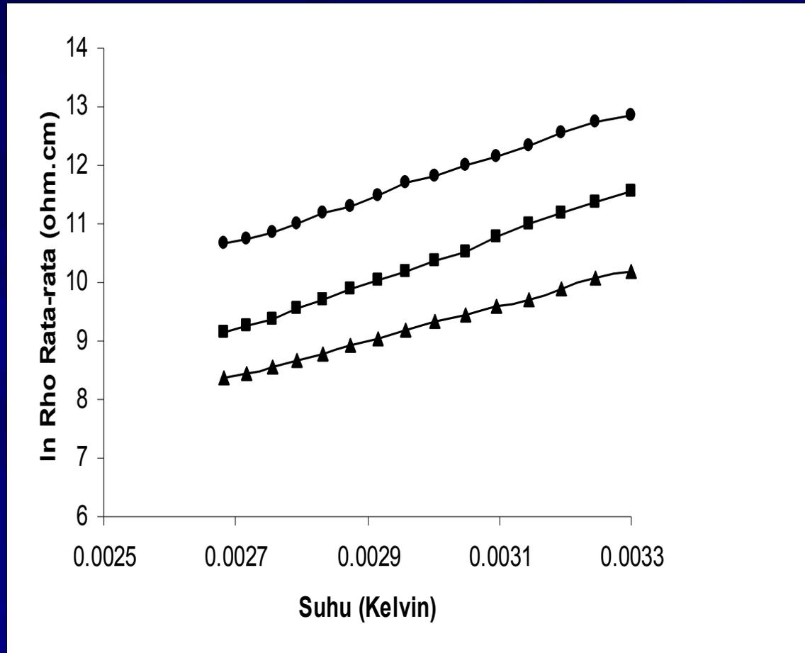
$\ln$  resistivity ( $\rho$ ) vs  $1/T$  of  $\text{SiO}_2$  added-  $\text{ZnFe}_2\text{O}_4$  ceramics.
