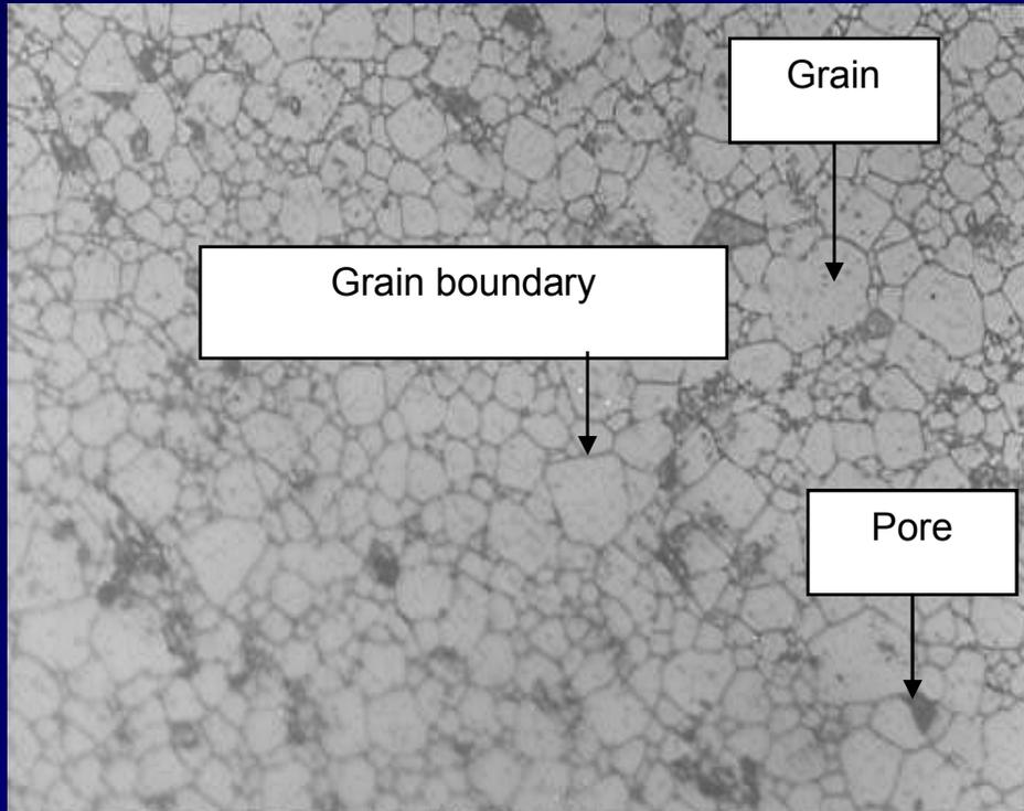
0 w/o SiO<sub>2</sub> sintered at 1200 C/2h/6 C/6 C
