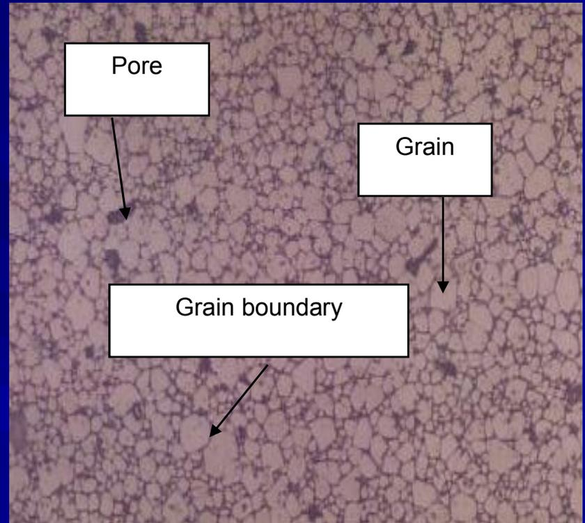
0.5 w/o SiO<sub>2</sub> sintered at 1200 C/2h/6 C/6 C
