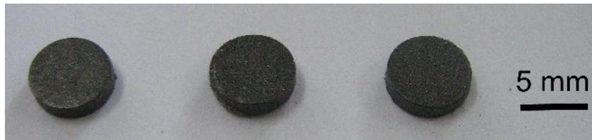
Fig. 1. Visual appearance of typical  $\text{SiO}_2$  Added- $\text{CuFe}_2\text{O}_4$  ceramic.
