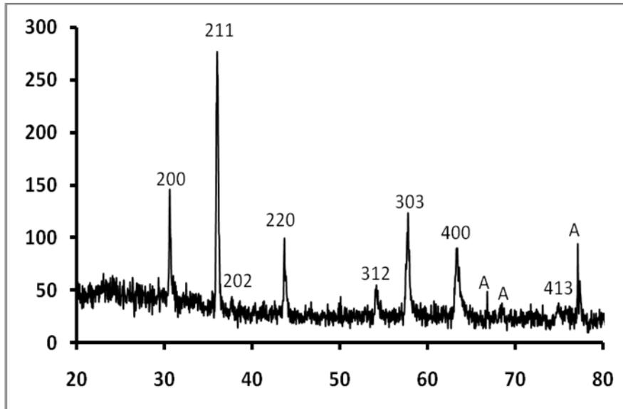
Fig.5. XRD profile of  $\text{CuFe}_2\text{O}_4$  based-thick film fired at  $1000^\circ\text{C}$  for 1 hr (with 5,0 % glass frit concentration)
