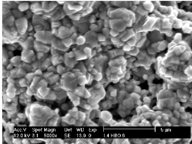
Fig.7 Microstructure of  $\text{CuFe}_2\text{O}_4$  based-thick film fired at  $1000^\circ\text{C}$  for 1 hr (with 2,5 % glass frit concentration)
