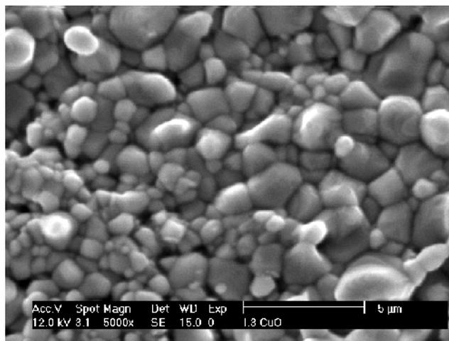
Fig.6 Microstructure of  $\text{CuFe}_2\text{O}_4$  based-thick film fired at  $1000^\circ\text{C}$  for 1 hr (without glass frit concentration)
