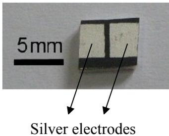
**Fig.2.** A typical thick film thermistor.
