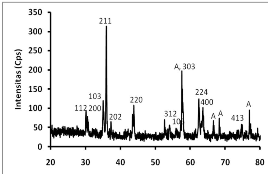
Fig.4 XRD profile of  $\text{CuFe}_2\text{O}_4$  based-thick film fired at  $1000^\circ\text{C}$  for 1 hr (with 2,5 % glass frit concentration)
