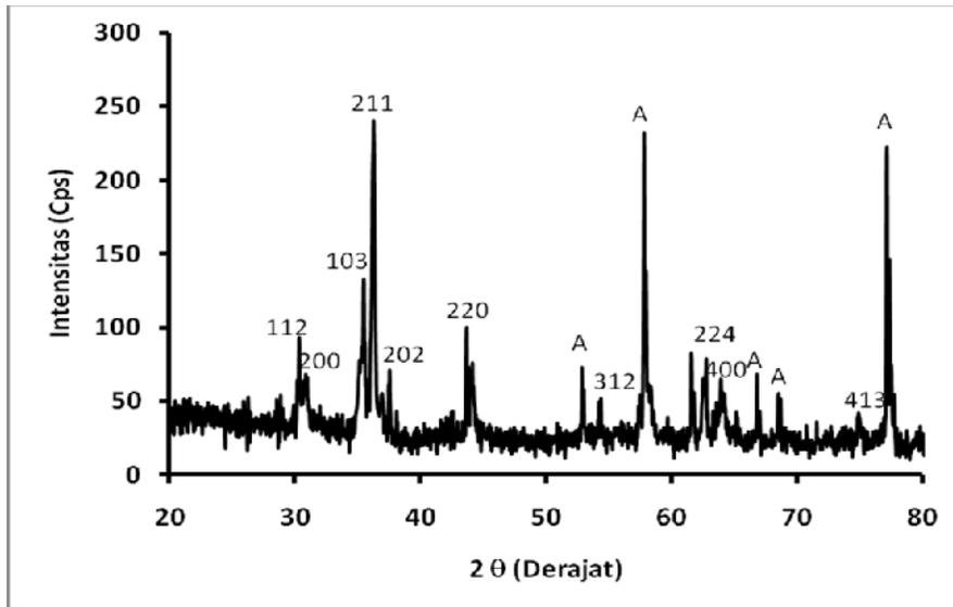
Fig.3. XRD profile of  $\text{CuFe}_2\text{O}_4$  based-thick film fired at  $1000^\circ\text{C}$  for 1 hr (without glass frit concentration)
