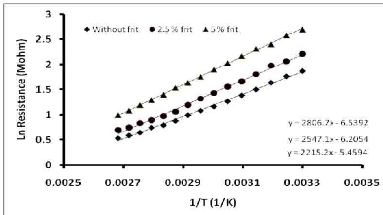
Fig.8. The relation between  $\ln$  Electrical Resistivity and  $1/T$  of  $\text{CuFe}_2\text{O}_4$  based-thick film fired at  $1000^\circ\text{C}$  for 1 hr (with : 0; 2,5 , 5% glass frit concentration)
