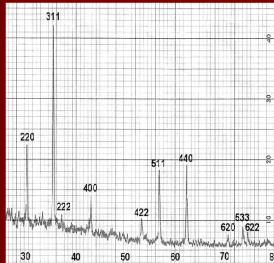
XRD profiles of ZnFe<sub>2</sub>O<sub>4</sub> based-ceramics.
