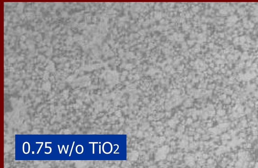
Microstructures of the ZnFe<sub>2</sub>O<sub>4</sub> based-ceramics.
