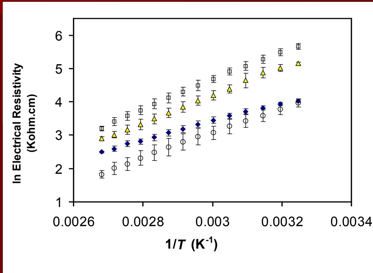
Ln resistivity ( $\rho$ ) vs  $1/T$  of TiO<sub>2</sub> added- ZnFe<sub>2</sub>O<sub>4</sub> ceramics.
