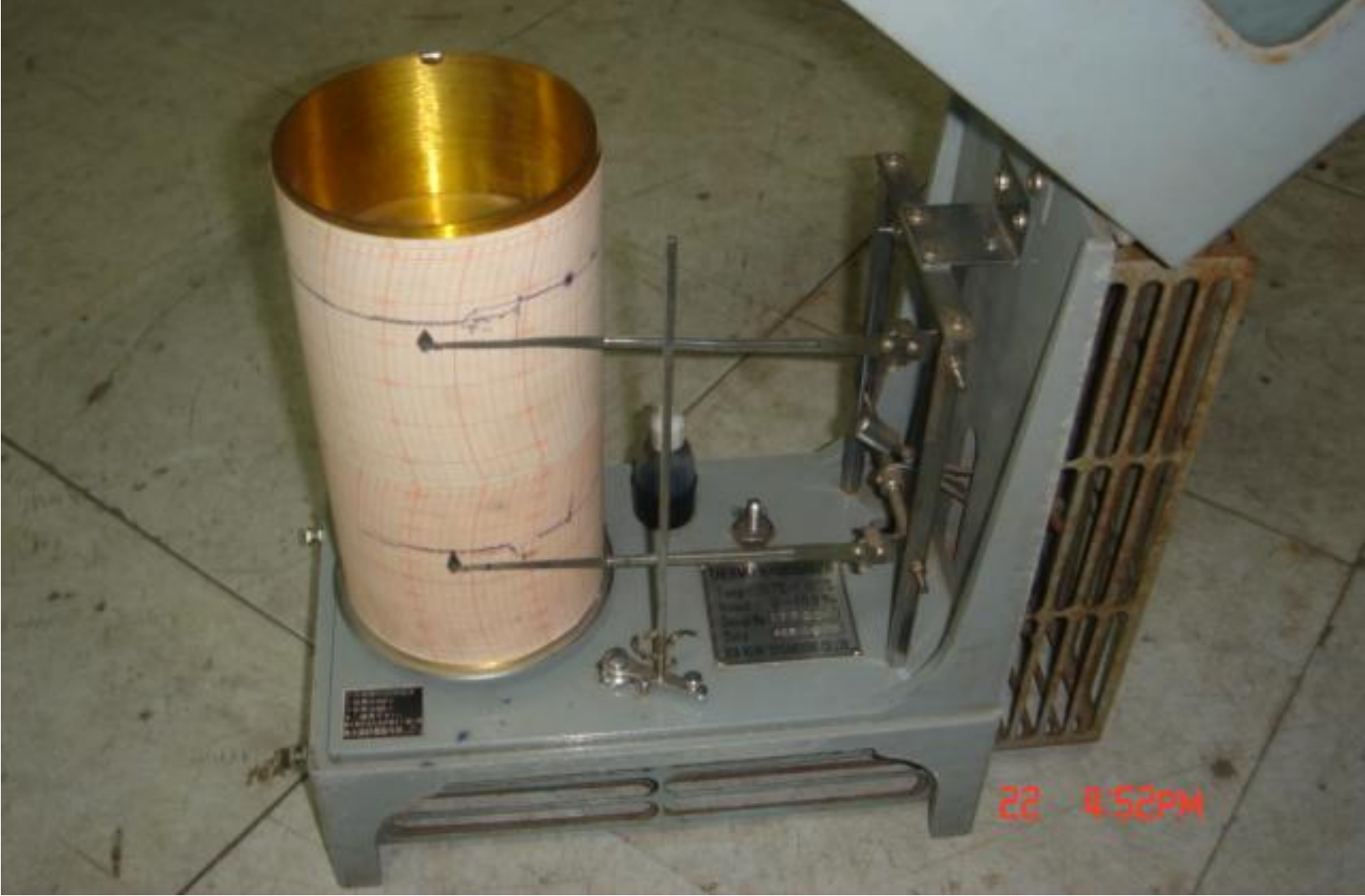
SISTEM PENCATAT THERMO HYGROGRAPH
